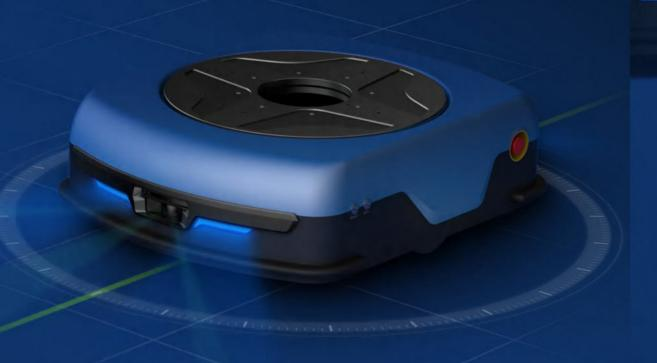
The moving robot is equipped with a new generation of QR code+inertial navigation / laser rader navigation / hybrid navigation to achieve precise positioning, more efficient and safer operation
