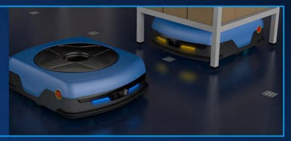
Equiped with anti-collision bar and obstacle avoidance radar, it is safer for both the people and facilities around.
